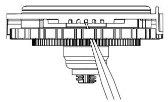
The drive cap assembly contains the drive cap, the main drive gear, drive cap spine, piston rod and various other parts that should not be dissembled in the field. The only replacement part on the drive cap assembly is the o-ring. Attached to the drive cap assembly is the main piston (downflow or upflow) and if a regenerant is used, a regenerant piston. Upflow if not applicable to EA, EE or EI control valves.
