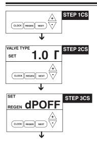
**STEP 1CS** – Press NEXT and ▼ simultaneously until TYPE appears on screen and release. Then press NEXT and ▼ simultaneously again for 3 seconds and release. If screen in step 2CS does not appear in 5 seconds the lock on the valve is activated.
