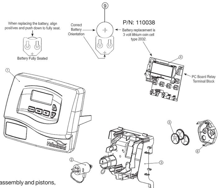
After completing any valve maintenance involving the drive assembly or the drive cap assembly and pistons, press and hold NEXT and REGEN buttons for 3 seconds or unplug power source jack from the printed circuit board (black wire) and plug back in. This resets the electronics and establishes the service piston position. The display should flash all wording, then flash the software version (ex: 214) and then reset the valve to the service position.
