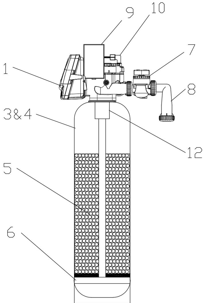
Compatible with the following regenerants or chemicals: Sodium chloride, potassium permanganate, sodium bisulfite, sodium hydroxide, hydrochloric acid and chloramines. For specific regeneration systems, contact factory.
